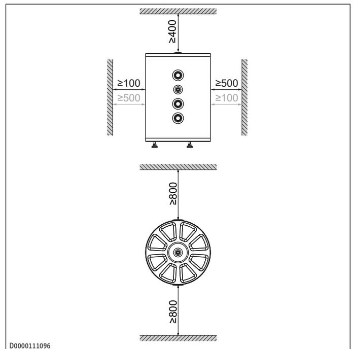
The minimum side clearances can be swapped between left and right.
